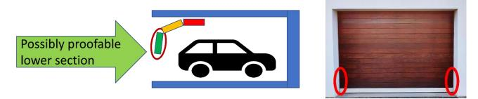
Do not install the horizontal and vertical seals overlapping. It could lead to friction problems.
